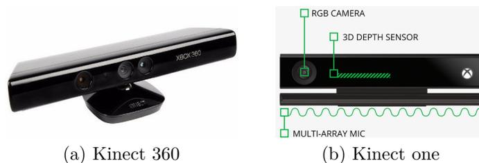
Figura 2 – Sensor Kinect
